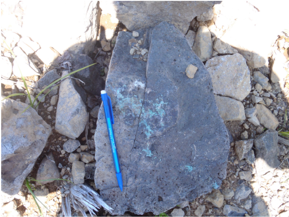
Figure 27: Sample 12979, 2,900 ppm Cu Feldspar phenocryst basalt, chalcopyrite seams
