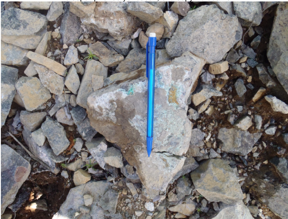
Figure 27: Sample 12979, 2,900 ppm Cu Feldspar phenocryst basalt, chalcopyrite seams
